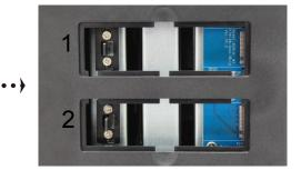
Important: Hold the SSD module by its edge, and do not touch the gold contacts.
