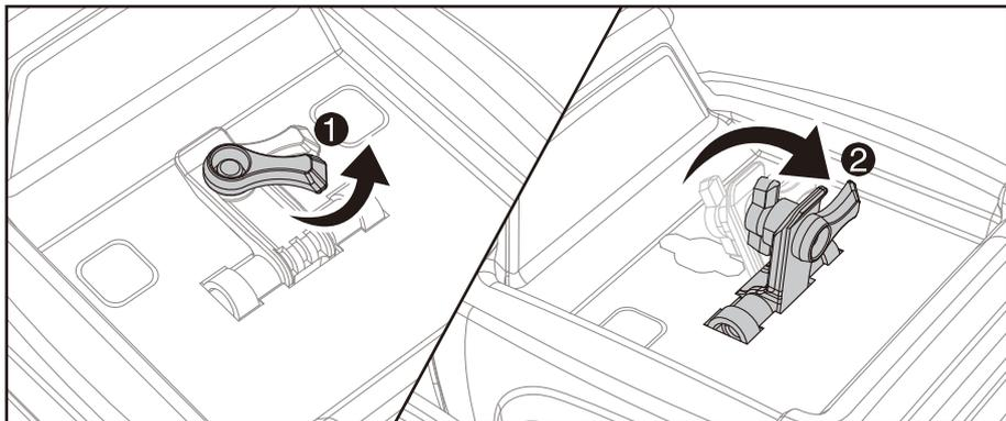
2. Insert the car shell into the front shock tower (as pic ③), then press the locking hook vertically down to the rear shock tower (as pic ④).
